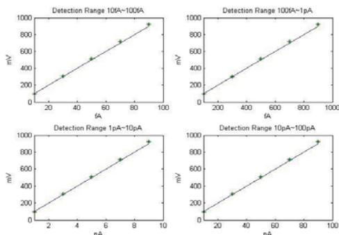
Fig. 7. Simulation results of readout circuit in 4 ranges
