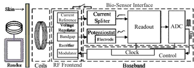
Fig. 1. Block diagram of the glucose sensor tag chip SoC
