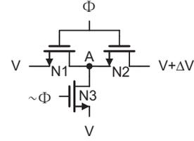
Fig. 5. Scheme of T-Switch
