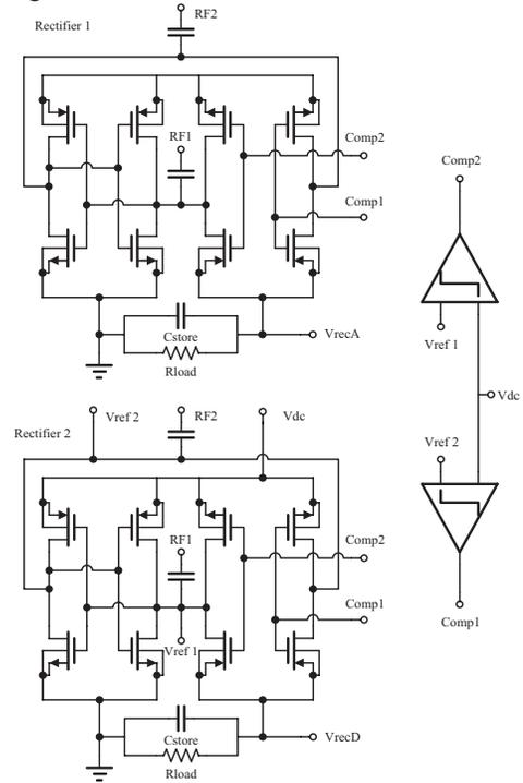
Fig. 3 Schematic of the rectifier
