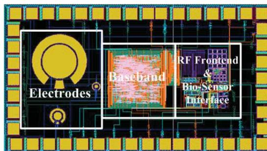
Fig. 8. Layout of the implantable bio-sensor tag chip
