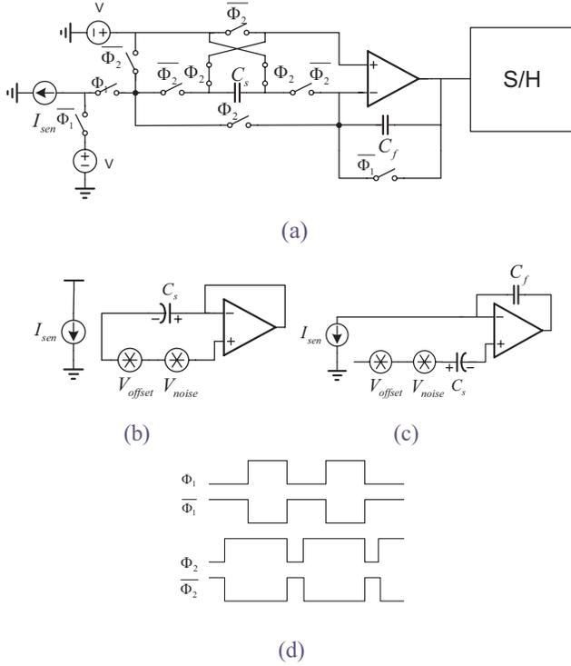
Fig. 4. Schemes of readout circuit: (a) Circuit scheme of the readout circuit (b) State of sampling in CDS (c) State of integration (d) The clocks
