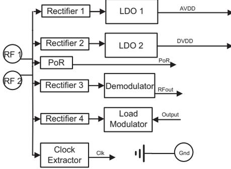
Fig. 2 Block diagram of RF-Front end
