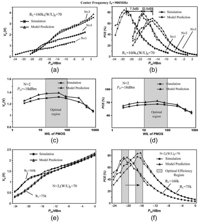
Fig. 3. (a), (c), and (e) are  $V_o$  of different  $N$ ,  $W/L$ , and  $R_L$ , respectively. (b), (d), and (f) are the PCE of different  $N$ ,  $W/L$ , and  $R_L$ , respectively.
