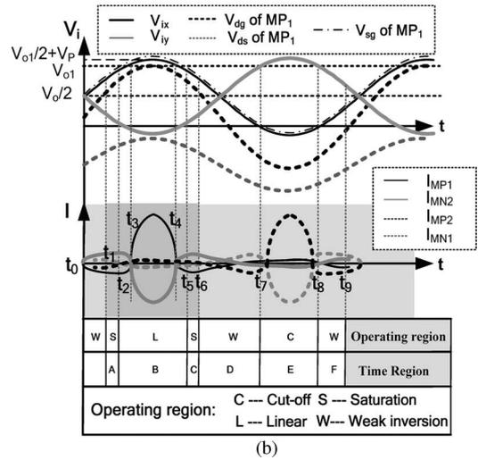
Fig. 2. (a) Single-stage topology of the rectifier. (b) Voltage and current curve of MOS transistors.
