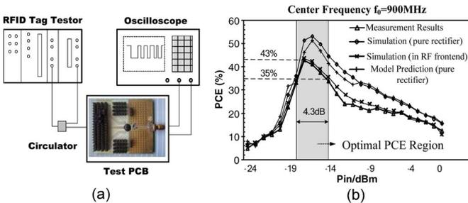
Fig. 7. (a) Test environment of the tag. (b) Comparison among test, simulation, and model results.
