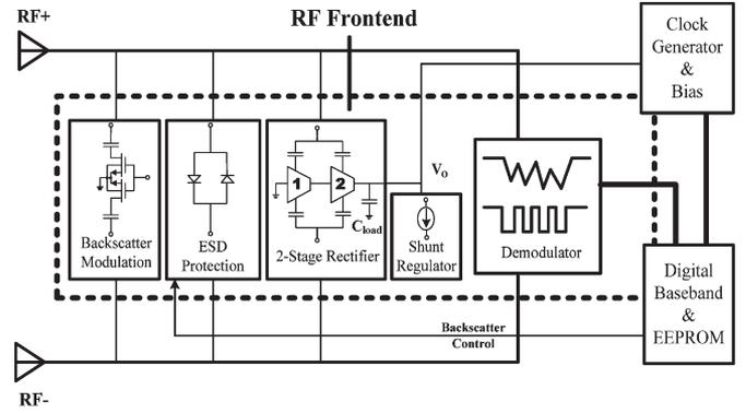
Fig. 4. Differential RF front-end architecture.
